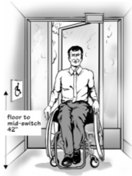
Power Operated Door at Entrance
